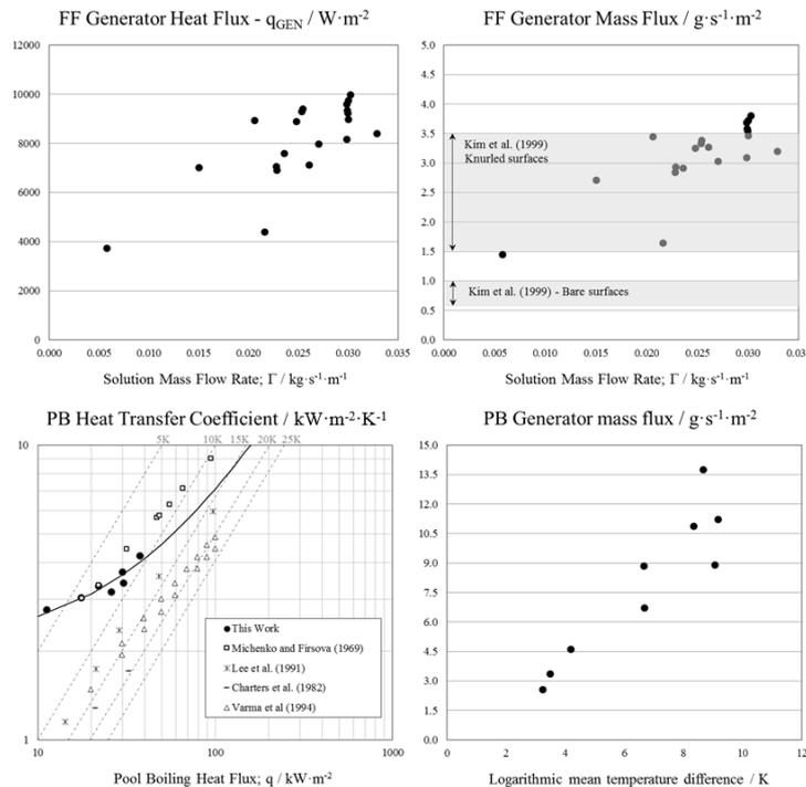
**Figure 2:** Falling film (FF) and pool boiling (PB) generators performance: heat and mass transfer fluxes.
