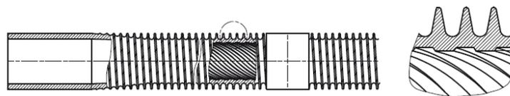
**Figure 1:** Scheme of the enhanced surfaces used for Falling-Film and Pool-Boiling Generators.
